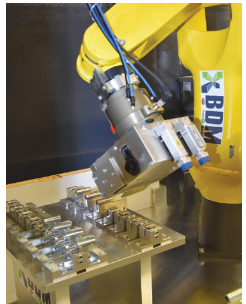
Robot-supported fitting of hinges
